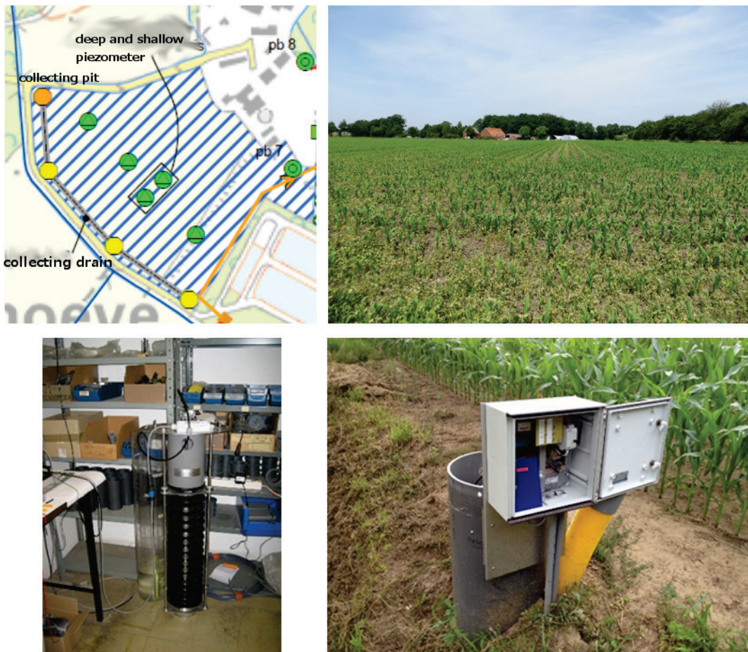
Figure 2: CAD experimental site Haaksbergen (5.5 ha area). Top left: setup of CAD and monitoring equipment (CAD-system; groundwater piezometers in green), top right: picture of the field in June 2013. Bottom left: mechanical drainage basis device installed within drainage collector pit. Bottom right: remote control unit with controlled drainage pit in the background.
